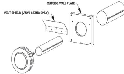
Does not include vent tube or cap. These items ship with unit.
